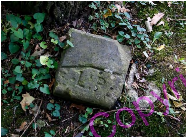
PBM 760. Grove Park Cemetery. SE9. Alongside fence at eastern end (at point where fenceline drops back east, the other side of which Elmstead Wood becomes Marvels Wood). The bent line represents boundary of Lee Parish where it changes course. Although stone appears to be at or near mapped location it has been turned clockwise 90 degrees, perhaps by adjacent grave digging..
